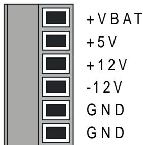
The board only requires +5V for normal operation. If however any additional PC/104 modules are fitted +/-12V may also be required. There is no on-board +5V to +/-12V converter. If required, +/-12 should be connected to the plug-in terminal block of PL17 as shown. The board typically draws 1A from the +5V supply with no power saving features active.
